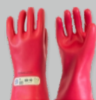
Gants isolants courts (28 cm) Classe 00 (500 V) Protection Arc-Flash ATPV 6 cal/cm 2 , APC 1 Réf: CG-00-R-28
