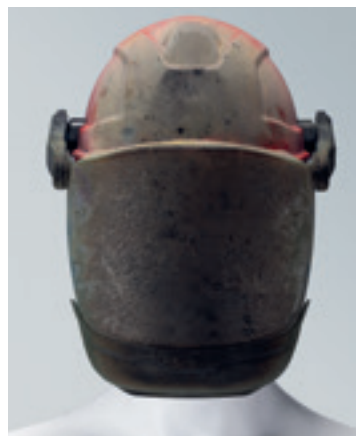
According to 7 kA short circuit electric arc
