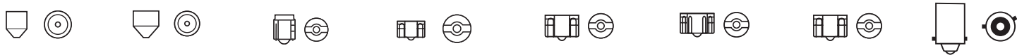
SV6 IEC 7004-5 SV8,5-8 IEC 7004-81 W2x4,6d IEC 7004-94 W2,1x9,5d IEC 7004-91 W3x16d IEC 7004-105 W3x16q IEC 7004-106 WX3x16d IEC 7004-105 BAX 9s IEC 7004-8
