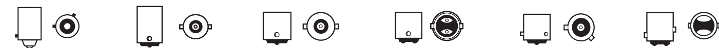
BAY 9s IEC 7004-9 BA 9s IEC 7004-14 BA 15s IEC 7004-11A BA 15d IEC 7004-11A BAU 15s IEC 7004-11A BAY 15d IEC 7004-11B
