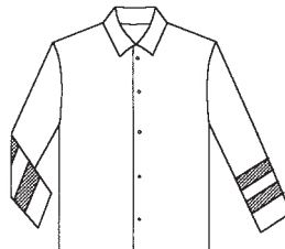
Two strips of reflective tape around the sleeve. VERSION: JX 252. 25 mm reflective tape. VERSION: JX 502. 50 mm reflective tape.
