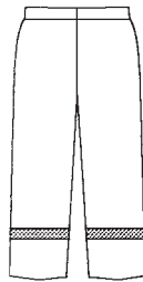
One strip of reflective tape around the leg. VERSION: BX 251. 25 mm reflective tape. VERSION: BX 501. 50 mm reflective tape.
